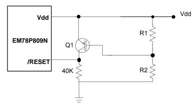
Fig 37. Residue Voltage Protection Circuit 2
